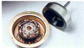
DC servo controlled Hall motor.
