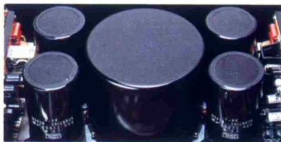
Huge power supply with toroidal core power transformer on SX-1250.
